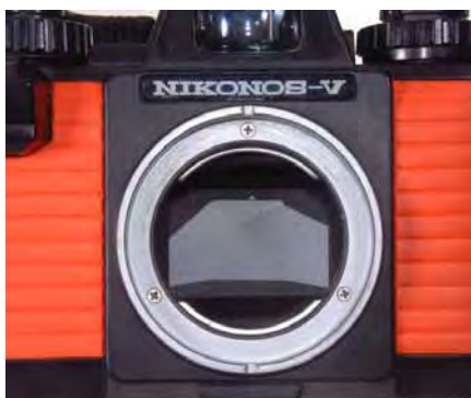
Take the lens off and look into the shutter blades. These must be clean and have no signs of slight corrosion
