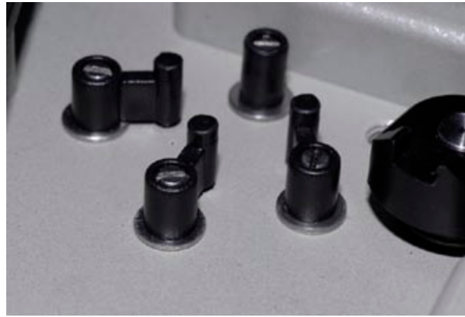
Extension required for multi selector control buttons – these are M3 stainless washers.
