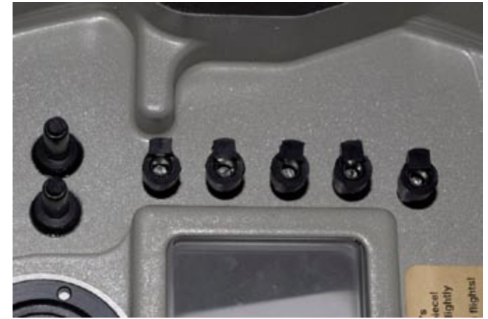
Push on extension pegs for buttons on left hand side of D300 review screen.
