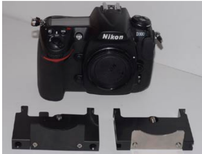
Re-designed D300 base plate and the original D200 base plate side by side with D300 in background.
