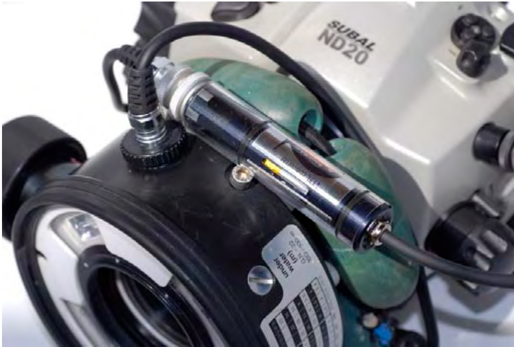
The Heinrichs Weikamp Nikon iTTL Converter installed on my Inon Quad flash and Subal ND20. Older flashguns like this will not communicate in iTTL but can be controlled on MTTL via the camera's exposure compensation dial. This extends the range of manual power settings significantly – down to 1/32 power at -5EV.
