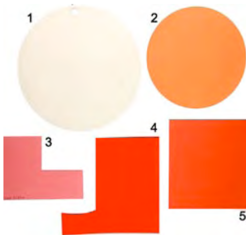
Figure 4. This is photo of some filters on a lightbox. Note that the strength of filter 1, a Lee 444 Filter - required to adjust a Inon at 5500K to a IkeliteDS125 equalling 4900 K is much, much weaker than other standard lens filters for underwater photography. It is also cheaper to buy as it is not made to optical quality. For information: 2 is Magic Filter, 3 is CC50Red, 4 is Wratten 22 and 5 is Auto-Magic Filter.
