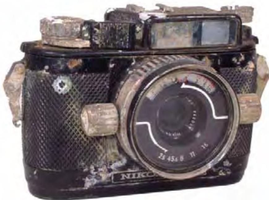
*The external appearance is usually a good indication of how hard a Nikonos 111 has been used. This one had been lost underwater for a year and then found again! The lens front port is clean because there was a close up lens attached.*
