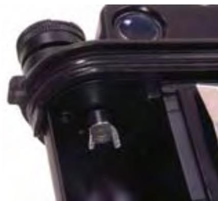
*Check that the inner silver rewind fork rotates freely when the rewind lever is down and that it engages when the lever is lifted and rotates with the rewind lever.*
