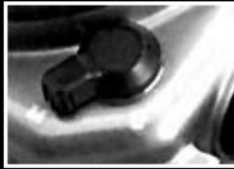
The focus mode selector operates the camera's M/S/C switch, which permits you to switch between manual, single servo, and continuous servo focus modes underwater.
