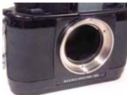
*If the O ring between the chrome lens mount ring and the outer body has not been regularly maintained there could be a build up of corrosion which eventually bridges the O ring.*
