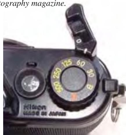
*Fire the shutter and watch how smoothly the wind on lever moves out. If it is at all sluggish the chances are the camera needs a service.*
