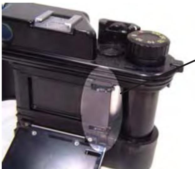
*Turn the shutter speed dial to 'R' and the film sprockets should rotate freely in either direction. set it to any other setting and they should click into place and only rotate when the film is wound on.*
