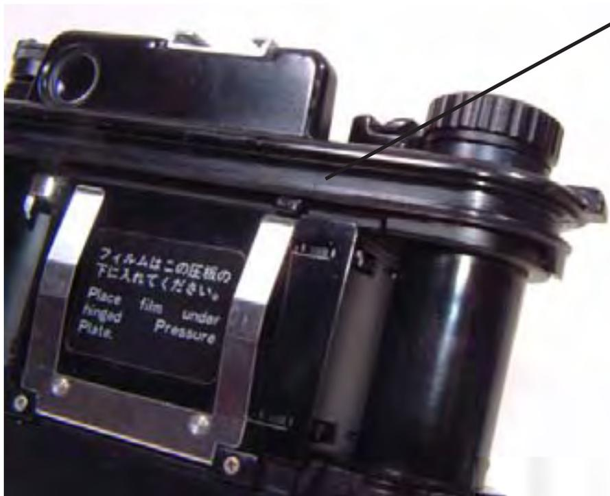
*Look out for a hairline crack in this area which has usually been caused by trying to remove the inner body with the lens still in place*
