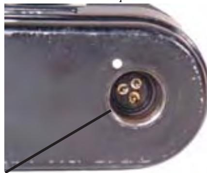
*Remove the flash port blanking plug and check the condition of the threads. There shouldn't be any corrosion in this area and the three contact pins should be straight and clean.*
