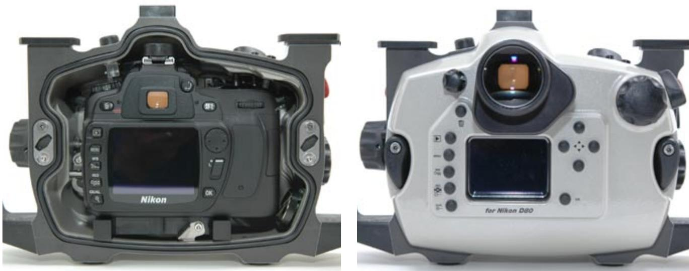
*As usual with Subal the camera is a snug fit in the housing. The main O ring seal is 4mm in diameter providing a large sealing surface area. The push button controls on the rear of the housing are smoother to operate and work accurately.*
