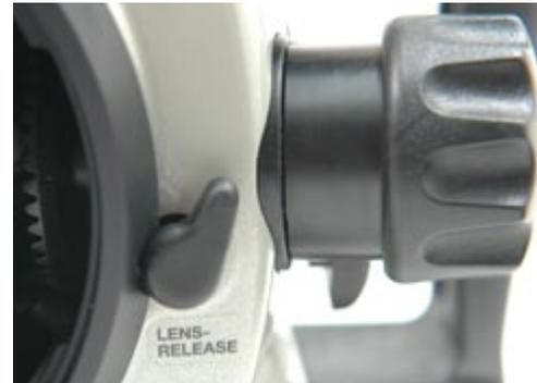
*The lens release lever allows lenses to be changed without dismounting the camera.*
