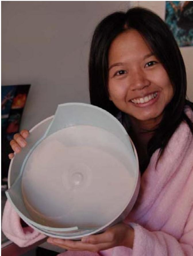
*Home-made Superdome cover made from 225mm UPVC end-cap and a short piece of pipe. With Darin Limsuansub!*
