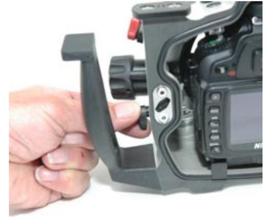
*Prior to mounting or dismounting the camera you have to pull out the MF/AF lever control.*
