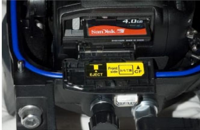
*It is possible to change the card (loading sideways) while the camera is locked in the housing. 2 Pins prevent accidental misalignment of the back when closing the housing.*
