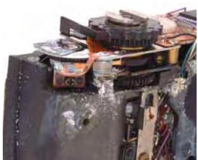
*Corrosion can clearly be seen around the frame counter assembly which also contains the main power contacts.*
