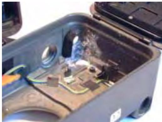
*It is only when the inner body is removed that signs of corrosion can be seen just under the frame counter window.*
