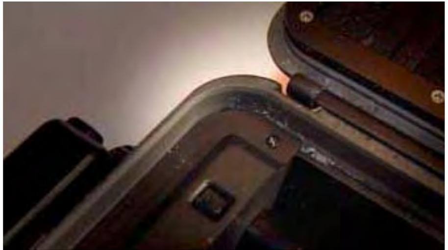
*Tell tale signs of corrosion . If you open the back with the camera pointing down, there is a strong chance that water will drop into the camera*
