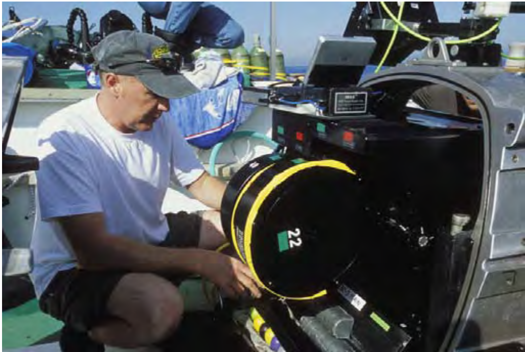
IMAX camera technician Stuart Macfarlane loads two reels of film into the IMAX® 3D camera—one for the right eye and one for the left eye—in California during the filming of the IMAX 3D film DEEP SEA 3D. Photo copyright© 2005 Warner Bros. Entertainment Inc. Photo: Drew Fellman
