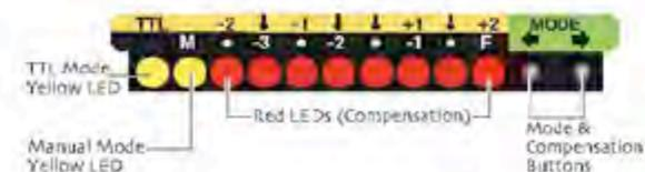
The Ikelite SLR-DC housings for Olympus have conversion circuitry and provide real Olympus TTL when used with Ikelite DS Substrobes but do not include the Flash Compensation Module.
