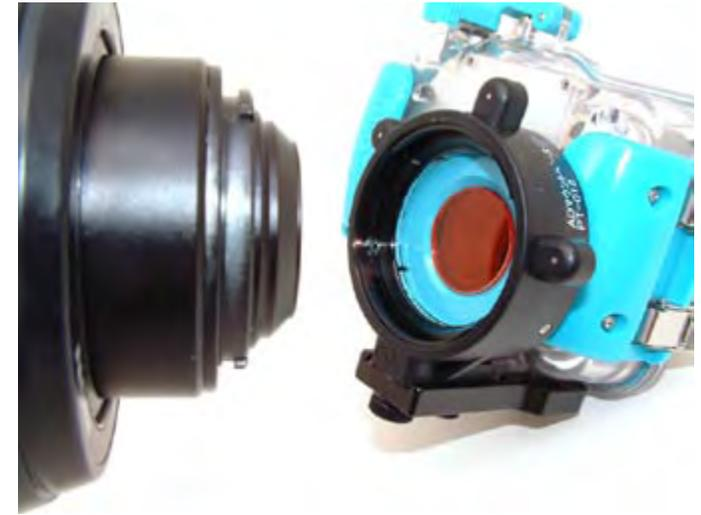
just enough space between the rear element of the UFL-165AD and the front port of the PT-012 to put a 27mm diameter filter. I achieved this by cutting out a circular disc from a larger UR-Pro filter but I understand they sell a 27mm filter in a screw mount which would do the same thing if it was taken out of the mount.
