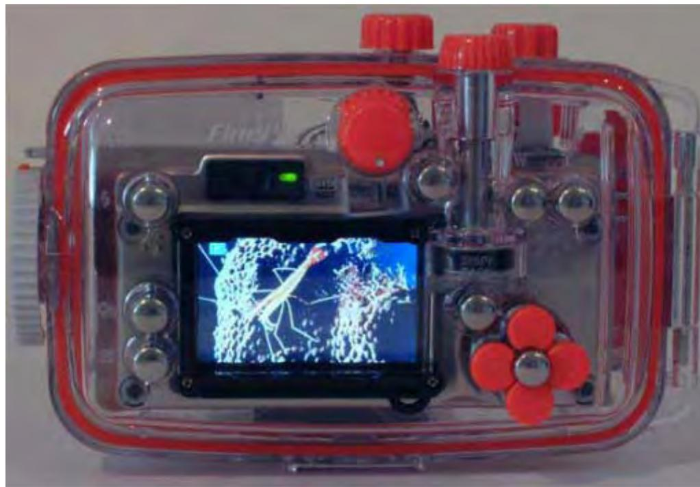
The built-in flash can be activated from the housing but there is now way of turning it off once it is opened either physically or from within the menu. Having been used to
