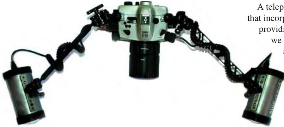
*My set-up for the telephoto photography underwater. Note how the strobes are as far out from the lens as possible and pushed forwards towards the subject.*
