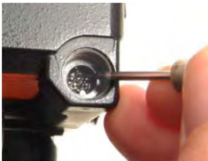
I didn't tell you to do this! Use a fine pointed device to push each of the two small sprung loaded pins up and down a few times and then blow the CL40 away with a blast of low pressure air.
