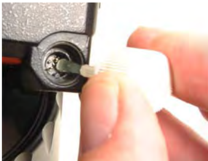
Diver's Best say don't do this but it has worked for me. Bear in mind that you haven't got much to lose because the only solution after this is to have a Nikonos repair technician replace the flash pin assembly from inside the camera and this is an expensive repair.
