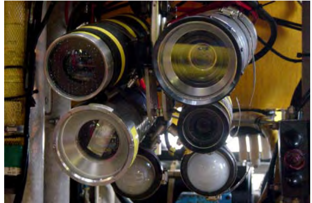
Kongsberg camera system on the pan and tilt arm. The camera housing is top right, and the flash tube is bottom left. Also mounted on the arm are colour video camera (top left), a low light video (bottom right) and a pair of video lights (right at the bottom),
