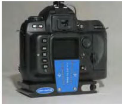
guides that keep the camera in exact position inside the housing. By pressing the metal release bar on the right of the camera tray, the camera and tray just pop out.
