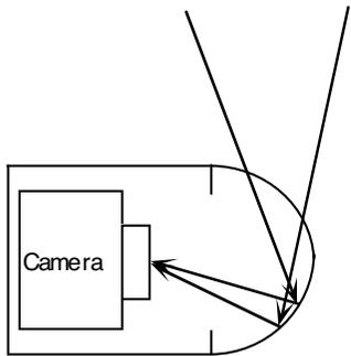
Dome ports are a simple and cost effective way of correcting most of the problems of refraction but can cause flare as light rays bounce from the inner surface of the dome and into the lens. This is internal reflection and becomes more of a problem the steeper the curve of the dome. The solution is to mask the surface of the dome not seen by the lens or use a lower profile dome
