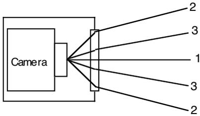
The light rays are refracted (deflected) at the air/water interface. The greater the angle of approach, the greater the refraction. Light rays (2) are refracted more than rays (3). Light ray (1) passes through the flat port at right angles so is not refracted, just slowed down
