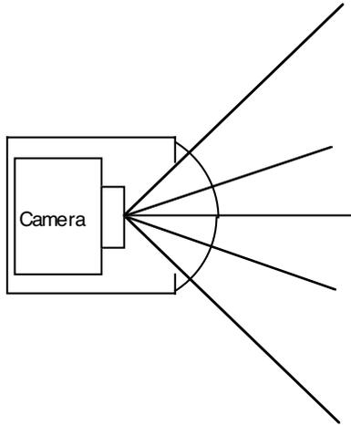
With a dome port, light rays are undeviated as they all pass the air/water interface at right angles. The result is a restoration of the angle of coverage of the lens
