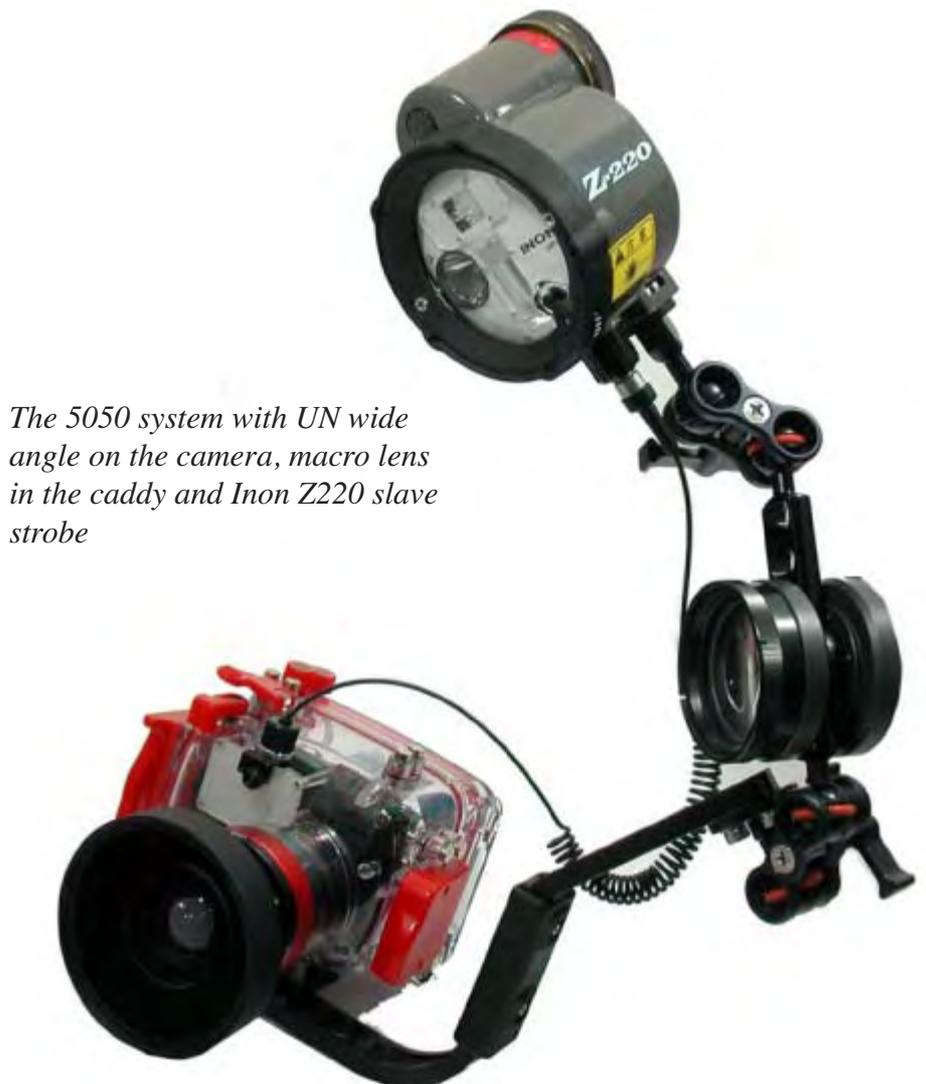
*The 5050 system with UN wide angle on the camera, macro lens in the caddy and Inon Z220 slave strobe*
