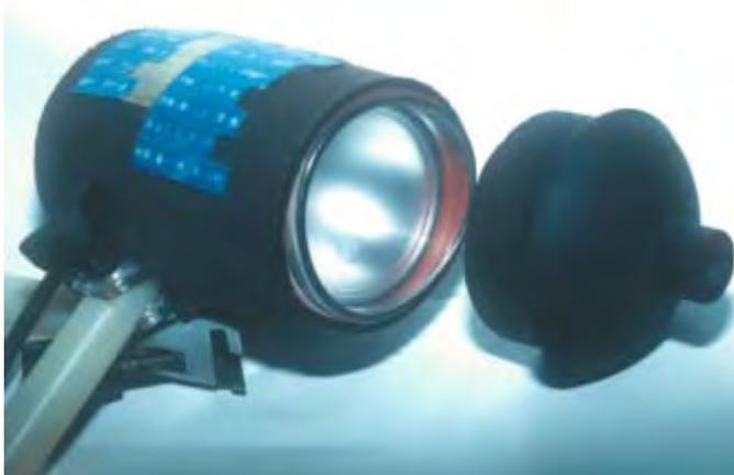
*Flash and snoot - You will need to light the foreground or macro subject very selectively to leave the remainder of the frame underexposed. Snoots can be constructed from a variety of odds and ends - this one comprises part of a watering can rose and a piece of drainpipe!*
