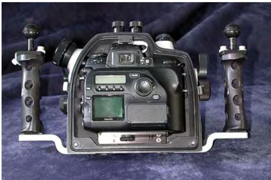
coated with a silver finish and a clear-coat on top of that, as well as anodized parts. The main seal is a single o-ring in a groove on the front of the housing and a face seal against the rear. To aid in aligning the rear of the housing when closing it up, Aquatica has fitted two stabbing guides to the bottom of the housing that fit into recesses in
