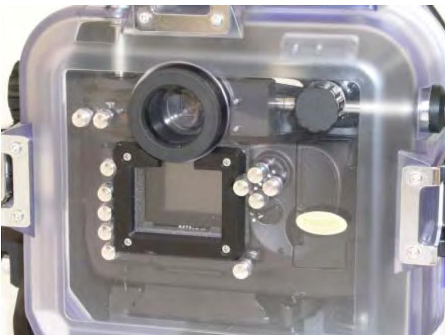
Disappointingly and similar to the NX100 housing the shutter release spring has not been improved, and is far too weak. The result is many unwanted frames or repeated frames. With the F100 housing it is easy to make a third turn in the spring to tighten it up, however, I had to resort in wedging a half inch (1.25cm) piece of eraser underneath it to achieve a similar result.
